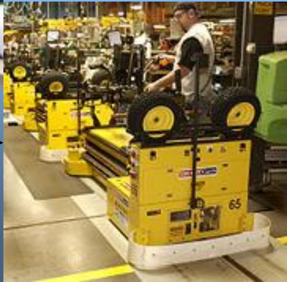
Light-duty assembly AGV →
