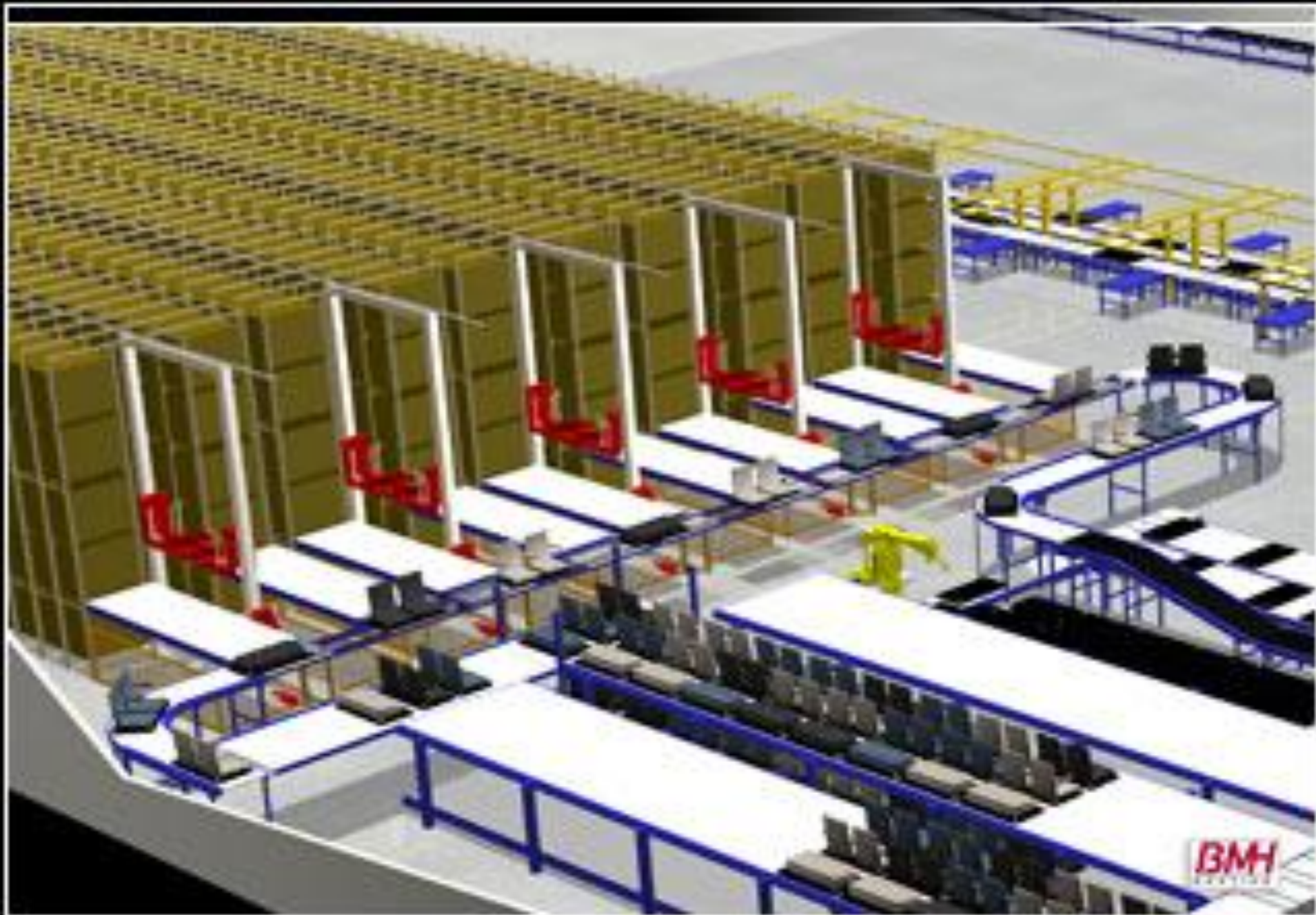
AS/RS Unit Load storage buffer for supply chain delivery
